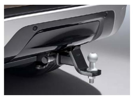
Towing System – Towing Receiver and Tow Hitch
