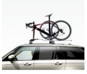
Fork Mounted Bike Carrier Roof mounted bike carrier provides a simple and secure fitting with the bicycle front wheel removed, ideally suited to lightweight bicycles and 'racing' wheels. A separate carrier is included for the front wheel. Easy to fit, lockable bike carrier that carries one bicycle per holder. A maximum of two holders can be fitted. \$550
